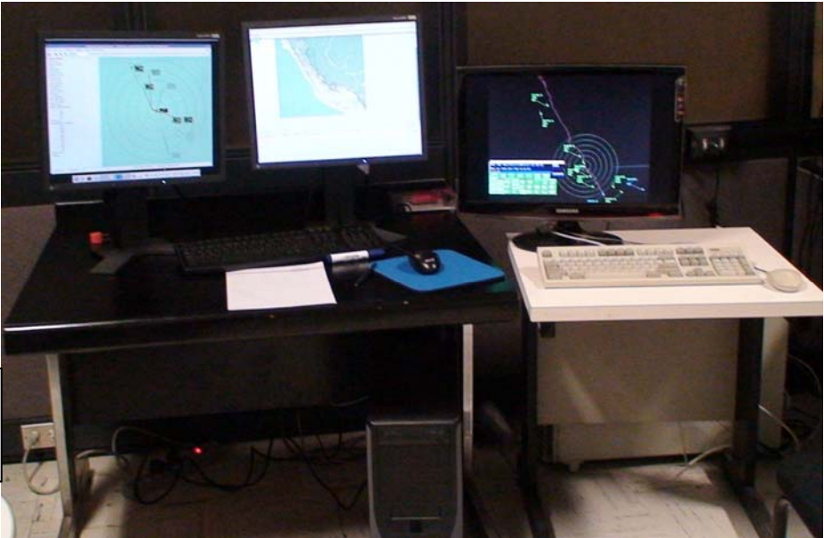
TSD (Technical Situation Display) terminal
